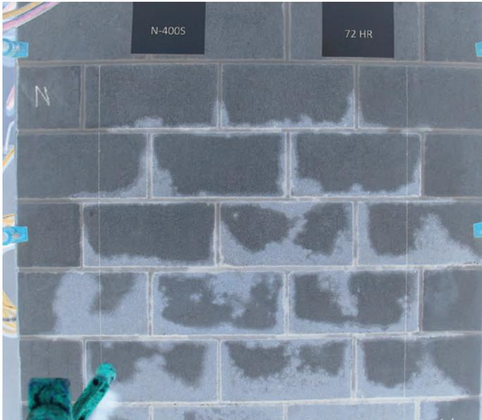
Untreated Mortar E514 wall after 72 hours.
